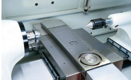
Bare cross slide with precision locator holes for custom applications.
