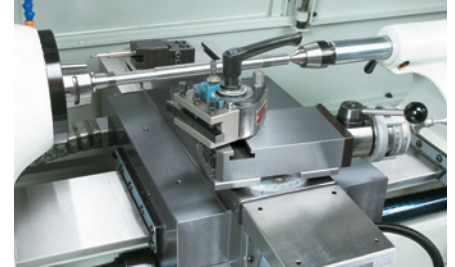
Lathe center in tailstock single tool on quick change tool holder on compound slide.
