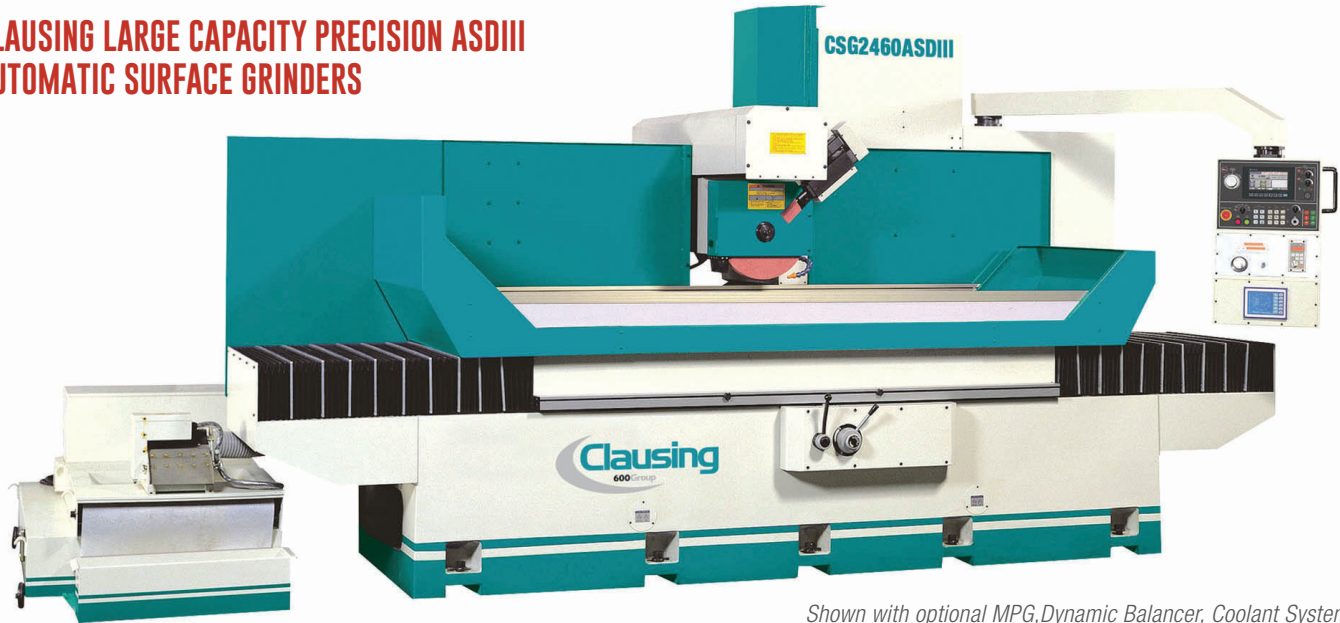
Shown with optional MPG, Dynamic Balancer, Coolant System with Auto Paper Feeding Device and Magnetic Separator
