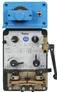
Clausing Installed Welder, Shear and Grinder. Welder Capacity: 1" Carbon Blades.
