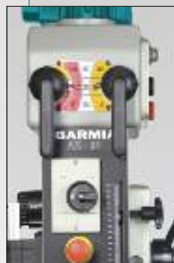
Head mounted speed controls for easy spindle speed setting
