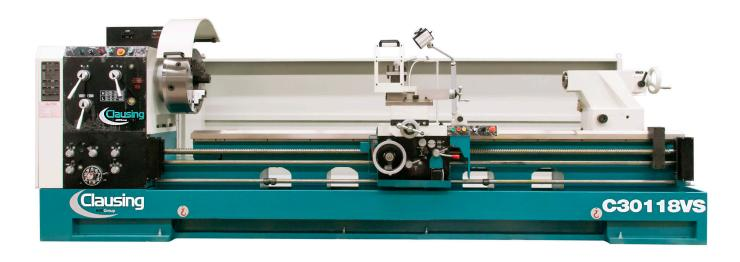
The C26 and C30 series large swing Variable Speed engine lathes are engineered to allow the accurate and efficient machining of large components. A wide range of optional accessories make these machines suitable for most industrial applications, including job shops, oil field, power utilities and ship building.
